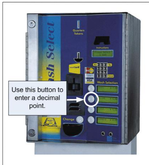
Figure 2. Entering the IP Address Decimal Point
