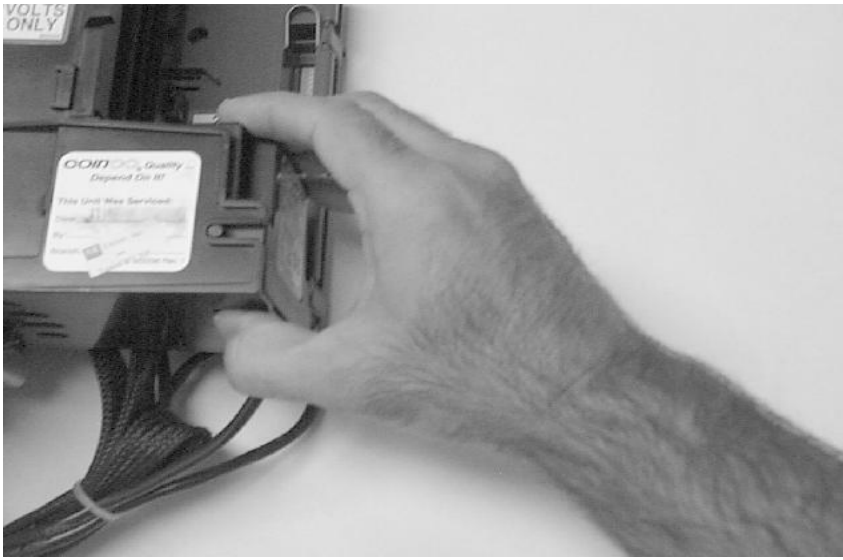
Figure 21. Removing Lower Housing
